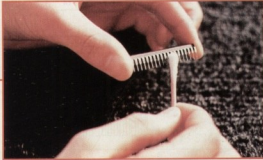
Using a cotton bud dipped in isopropyl alcohol, wipe both sides of the legs of the IC to remove any contaminants. (Usualty coffee!) This can occasionally bring success.
